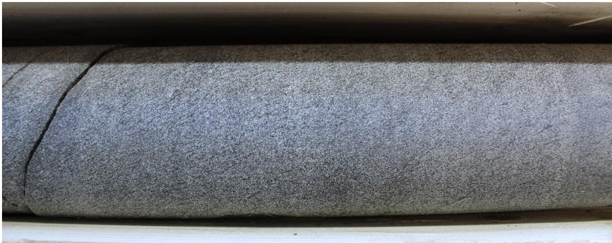
Figure 12 Intermediate volcanic (PONT056 30.30 m)
