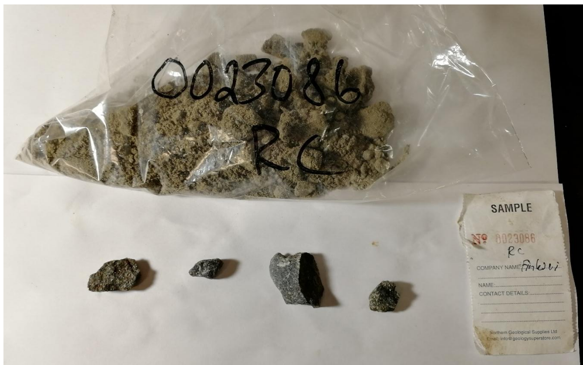
Figure 47 Bedrock chip material recovered with GM50. The larger chips are washed and logged. Also shown are the sample tag numbers assigned by GTK to the sample on collection.
