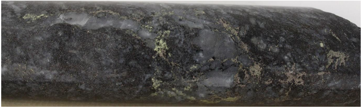
Figure 20 Pyrrhotite and chalcopyrite mineralisation associated with fragmented quartz veins in Diorite. (PONT053 70.90 m)
