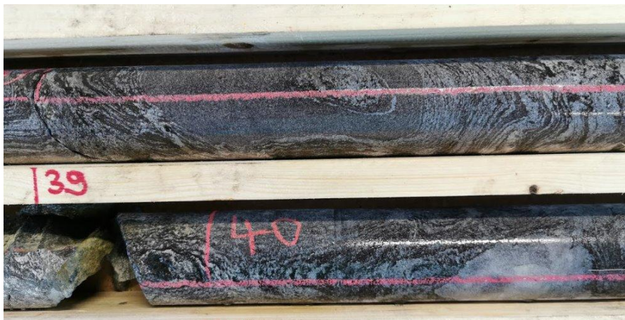
Figure 10 Biotite Gneiss, a biotite rich paragneiss (PONT030 approx 40m)
