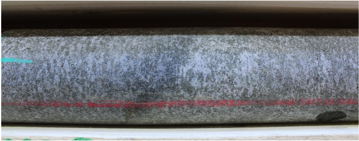
Figure 14 Medium grained Diorite (PONT057 89.25 m)
