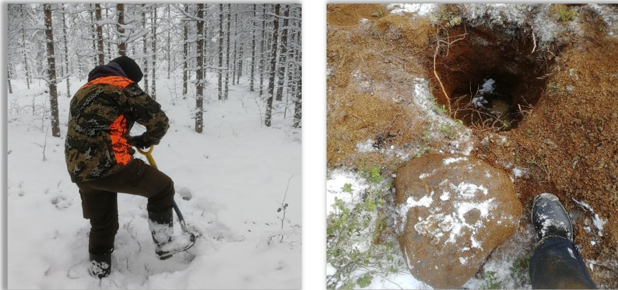
Figure 33 Surface till sampling using a shovel to dig a hole from which a sample is taken from the desired substratum (C-Horizon). In places the Horizon was quite thick.
