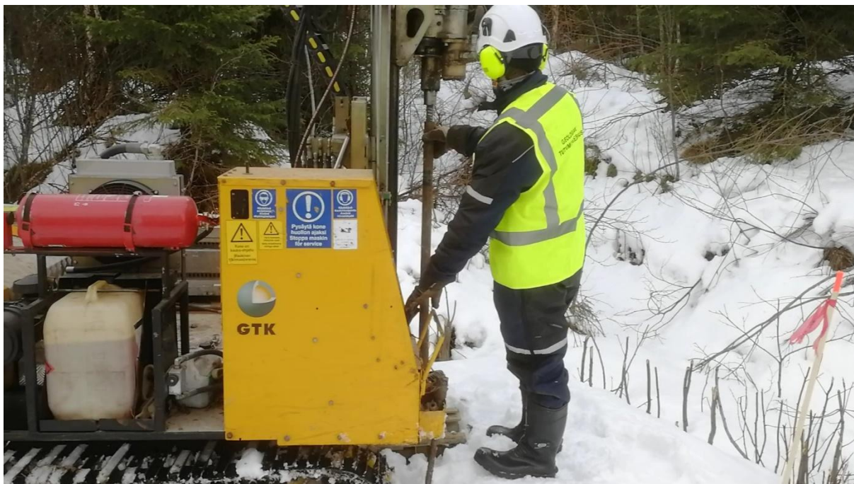
Figure 39 GTK GM50 and operator at a BOT sampling site
