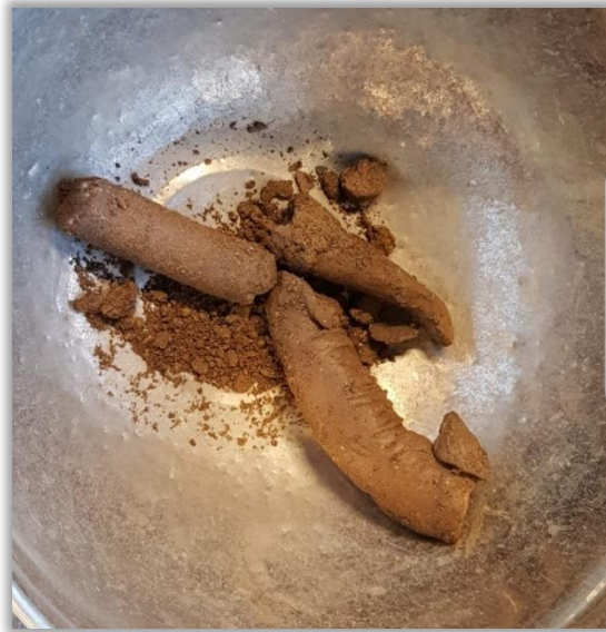
Figure 36 Base of Till (BOT) material in metal bowl for disaggregation and drying prior to sieving
