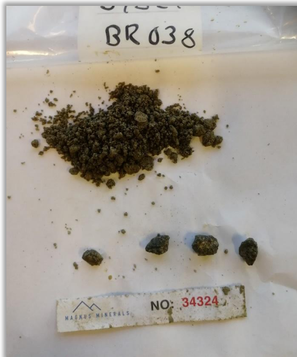
Figure 37 "Bedrock" chip material recovered with Cobra. The larger chips are washed and logged. Also shown are the sample tag numbers assigned by Magnus Minerals to the sample on collection.
