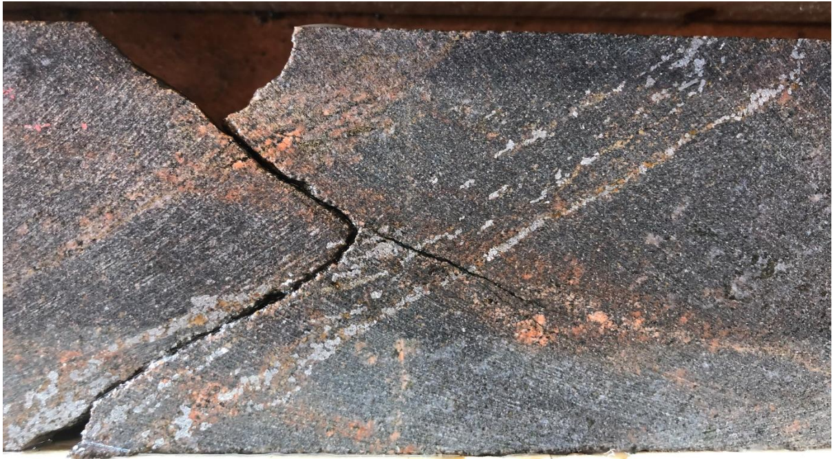
Figure 18 Disseminated and stringer arsenopyrite mineralisation in a deformed and oxidised Diorite. (PONT052 67.25 m)
