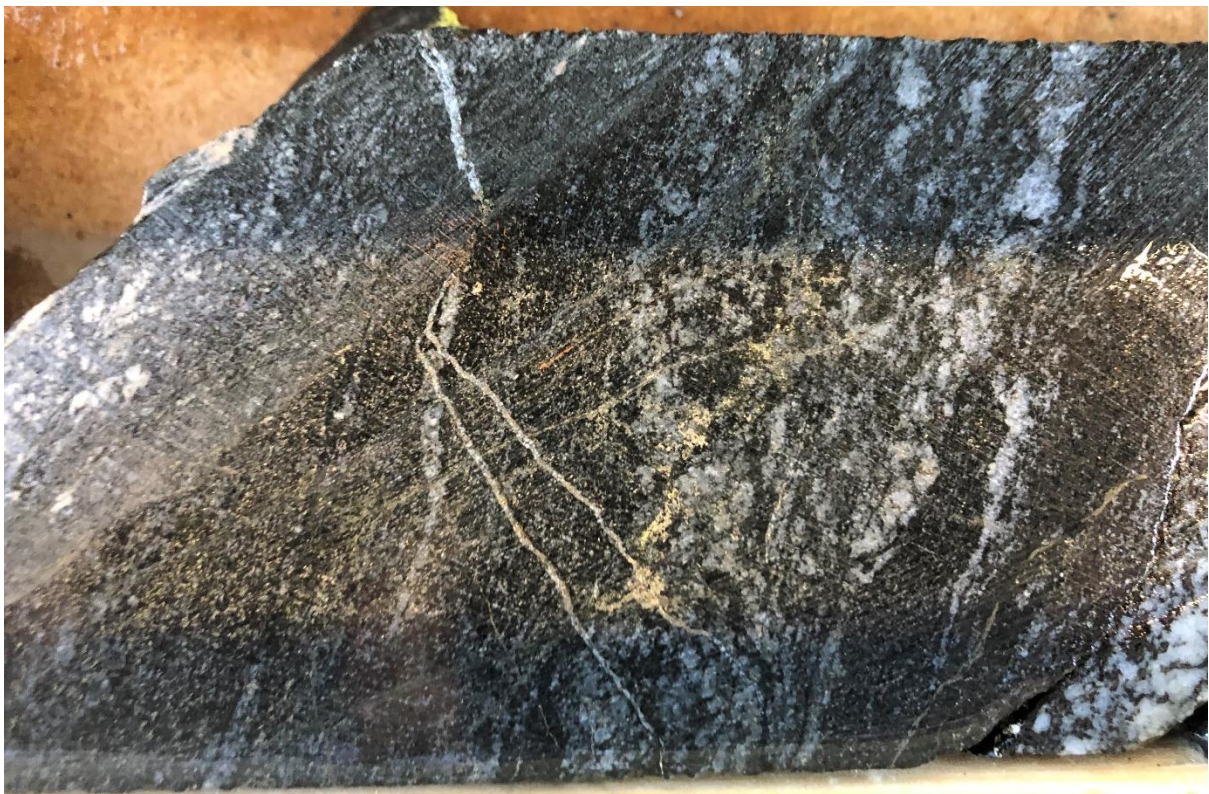
Figure 19 Disseminated chalcopyrite in an altered, veined and sheared Diorite. (PONT040 113.85 m)
